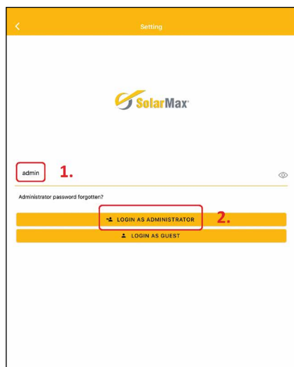
Fig. 23: Login to the inverter
